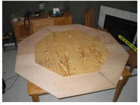
To center the little octagon on the big one I snapped chalk lines between all the corners. To double check it's placement you can also measure to be sure the race track is approx 11" all the way around. Next up was laying out the location of the cup and chip holders. I decided to put the cup holders on the left hand side of the player because most people are right handed and I didn't want
