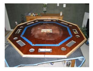
You could apply poly to the whole larger octagon but why only the race track will be exposed. I applied the first light coat of ploy with a good brush and let it dry 6 hours. I then sanded the poly with 220 grit sand paper and applied another light coat. After 2 light coats I decided this is going to take for ever to build up and applied a heavy coat of poly. Big mistake when it dried I ended up with
