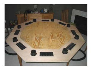
With the holes cut it was time to stain the wood. Before staining I sanded the wood down with 220 grit sand paper. This makes the wood smooth but it also remove the chalk lines I snapped earlier. I let the stain sit for 40 minutes and the whipped the excess off.
