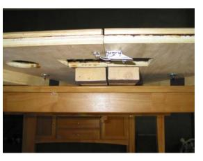
Since I am building a table top that is going to hang over the edges of my table I wanted to give the boards more support so it wouldn't bend over time. Simple solution was to screw 2X4s to the bottom of the large octagon. When placing them, be sure to avoid the cup holders and the holes you drilled for the tee nuts. Also be sure you don't put any screws in the race track area or they will be visible.
